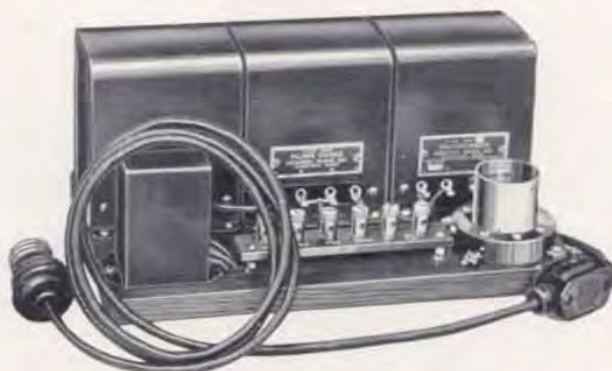
Above illustration shows a Raytheon "B" battery eliminator constructed of all General Radio parts. Note neat arrangement of parts and compactness.
